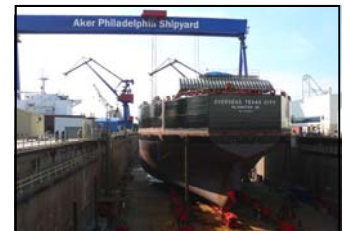
Hull 009 being skidded forward
